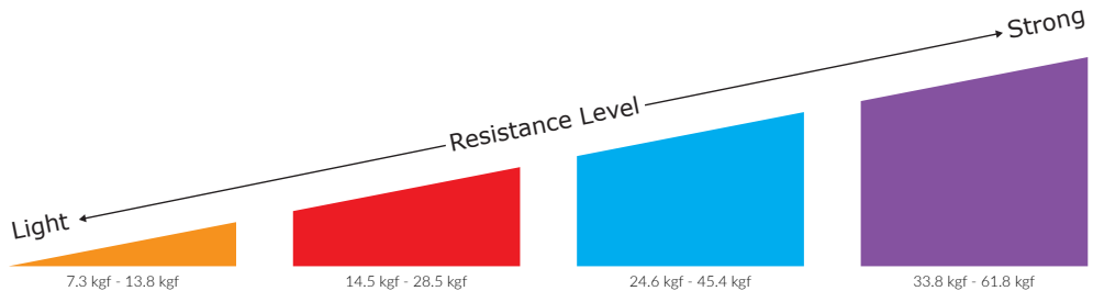
Typical Pull Force Chart With An Elongation Percentage of 100% to 300%
